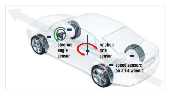
ESC is an extension of ABS, which has speed sensors and independent braking for each wheel. Additional sensors monitor how well a vehicle is responding to a driver's input.
