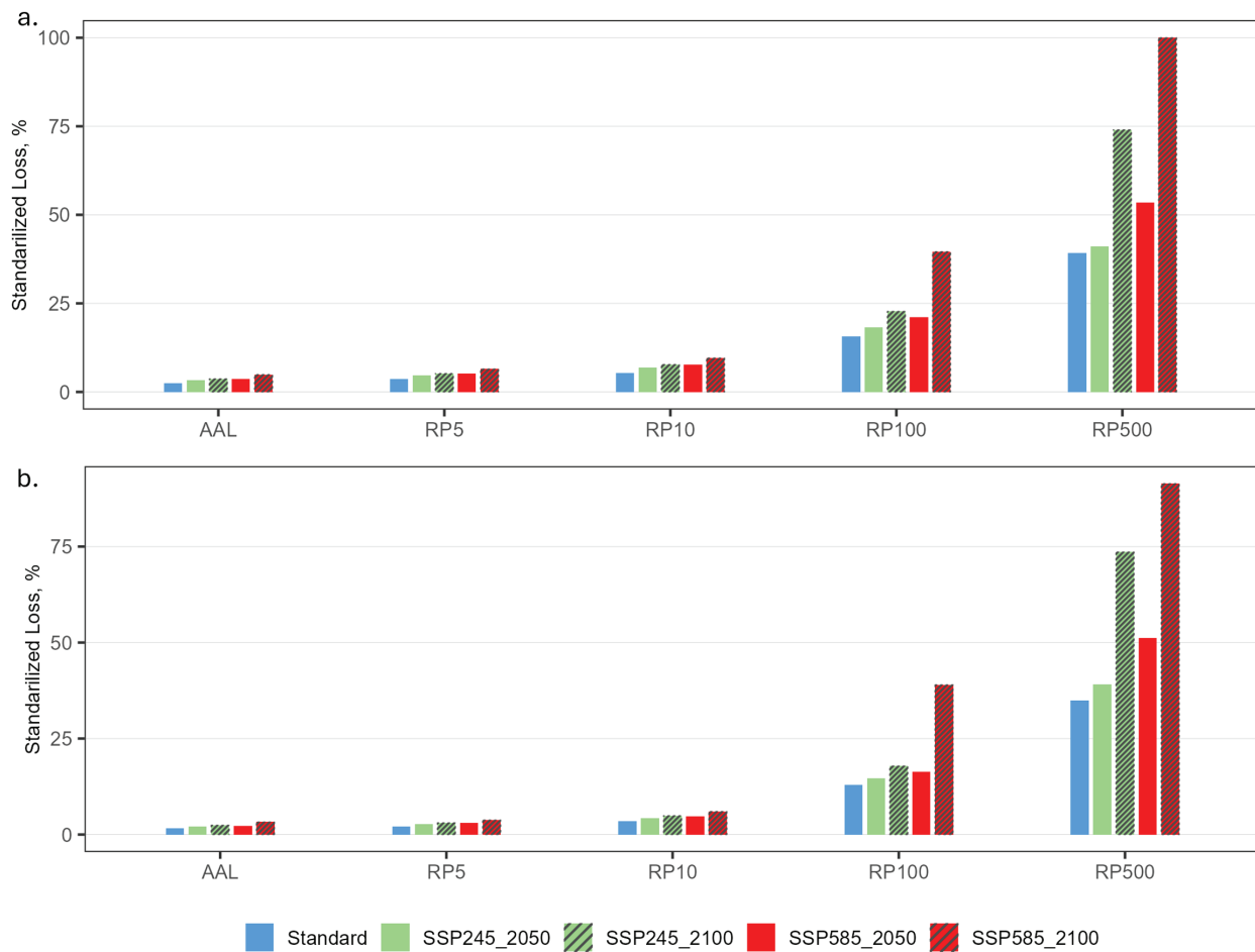
Figure 10. a. Aggregate loss; b. Occurrence loss increases in SSP2-4.5 and SSP5-8.5 compared with the current climate condition.
